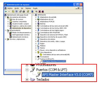
1. Using the Control Panel go to the "Components Manager", then look for the "Ports (COM & LPT)" section. If the APS Master Interface was correctly installed you will find it there.
