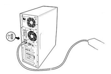
1. Connect the APS Master Interface to your computer using an USB Cable.
