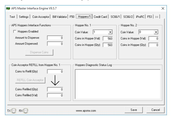
If you want the APS Master Interface Engine to use the Coins Hoppers to dispense change, first you need to check the "Hoppers Enabled" checkbox under the "Hoppers Functions" section, then you need to select the "Coin Value" that you will be using under the "Hopper No. X" sections. If for any reason you want to disable an individual hopper but still using the other you can do it by selecting a "Coin Value" of "0".
