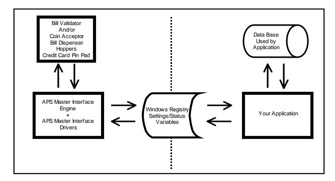
Windows Registry values are used to store APSMI Engine settings such as General Settings for Bill Validator and Coin Acceptor, type of bills to accept, value of the type of bills accepted, type of coins to accept, enable/disable delivery of change, etc.
