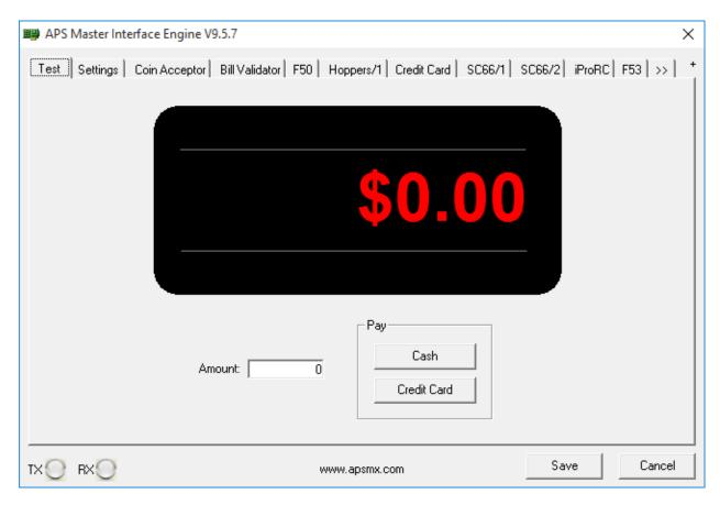
The APSMI Engine Console is divided into 12 sections. Test Console and Settings are used for all the payment devices. Each additional tab is related to the connected equipment. In the following chapters we will describe in detail every single one.
