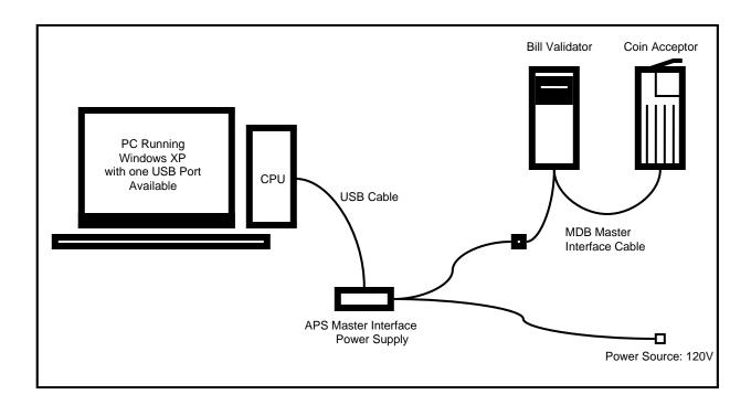
The APSMI is powered up by the USB connection. An additional External Power Supply is required to power up the Bill Validator and/or Coin Acceptor.
