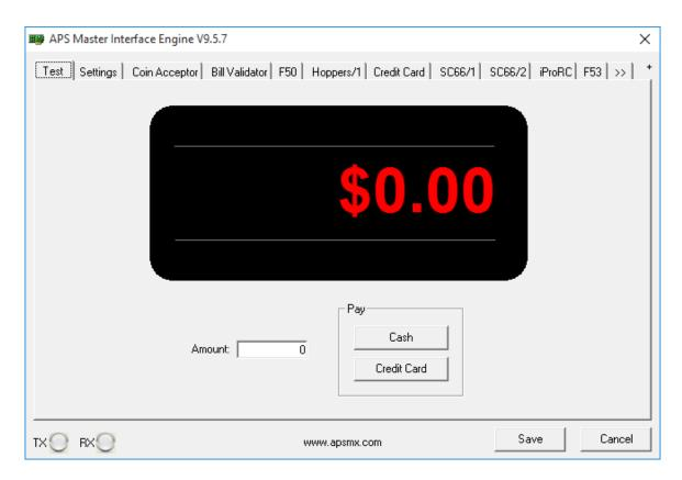
To test your equipment you just need to type the Amount of money to be charged in the "Amount" textbox, then click the "Cash" button. The APSMI Engine Console will activate the Bill Validator and/or Coin Acceptor so you can start inserting the money.
