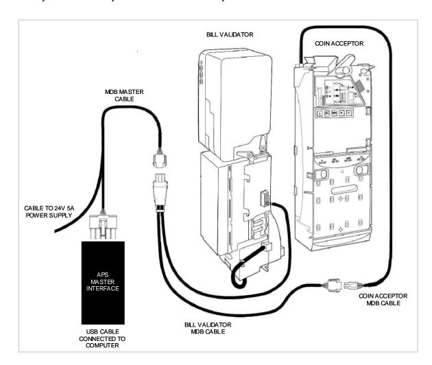
Some equipment have to be configured to support the MDB protocol. Please make sure your equipment meet this requirement before connecting it to the APSMI. If your equipment is already included in the list of equipment tested by APS (Chapter 2.5) and you need additional information on how to set it up, please feel free to contact us to support you on this task.
