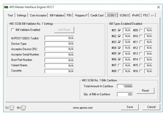
The SC66 is connected directly to the PC so it doesn't require the APS Master Interface. It can be connected to a USB or RS232 Port. The type of port is defined by the Bill Validator version.
