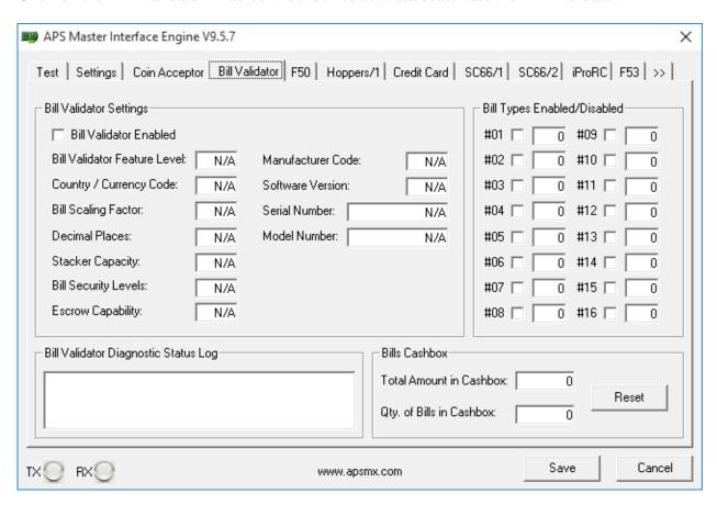
MDB protocol requires Bill Validators to send the "Bill Type" inserted by the user when the equipment is operating. There are 16 different types of bill supported by the MDB protocol.
